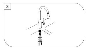
Remove the 2 screws from locking nut .From under the sink,install the rubber washer,steel washer,and locking nut onto the shank Tighten the locking nut with a basin wrench or socket tool and install the 2 screws to secure the faucet in place.
