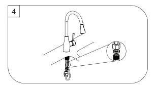
Install counter weight onto pull out hose.Connect the pull out hose to water inlet tube.Be sure to install rubber washer. Do not overtighte the connection.
