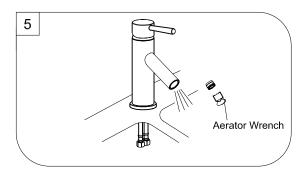
Important: After installation is completed. Remove aerator then turn on water supply and allow both hot and cold water to run for at least one minute each. While water is running, check for leaks. Reinstall Aerator. Your new faucet is now ready to use.
